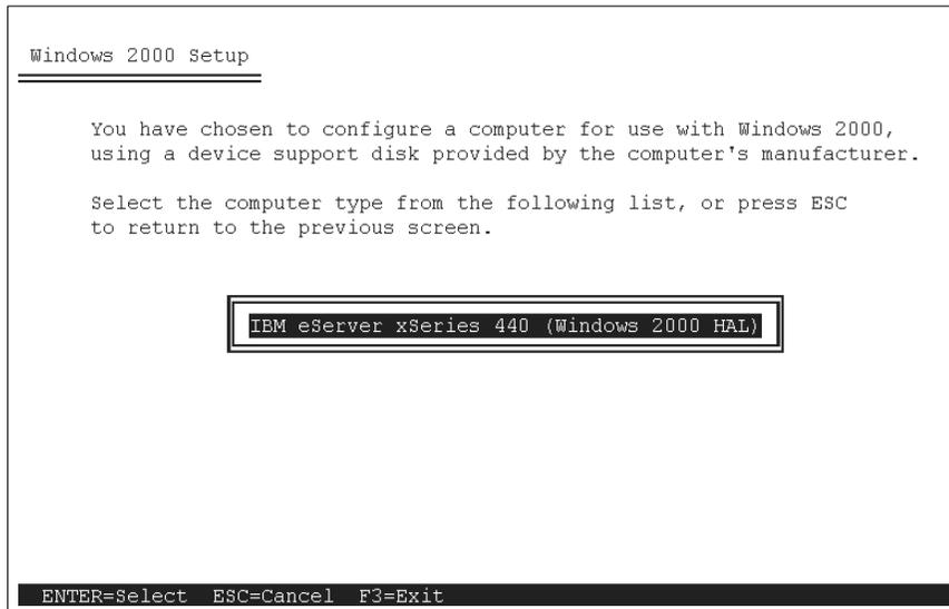
Figure 4-4 Selecting computer type from custom HAL disk
