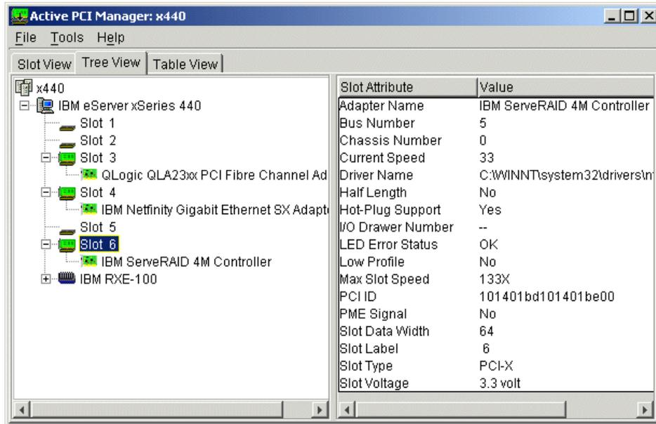
Figure 5-16 Incorrectly arranged adapters
