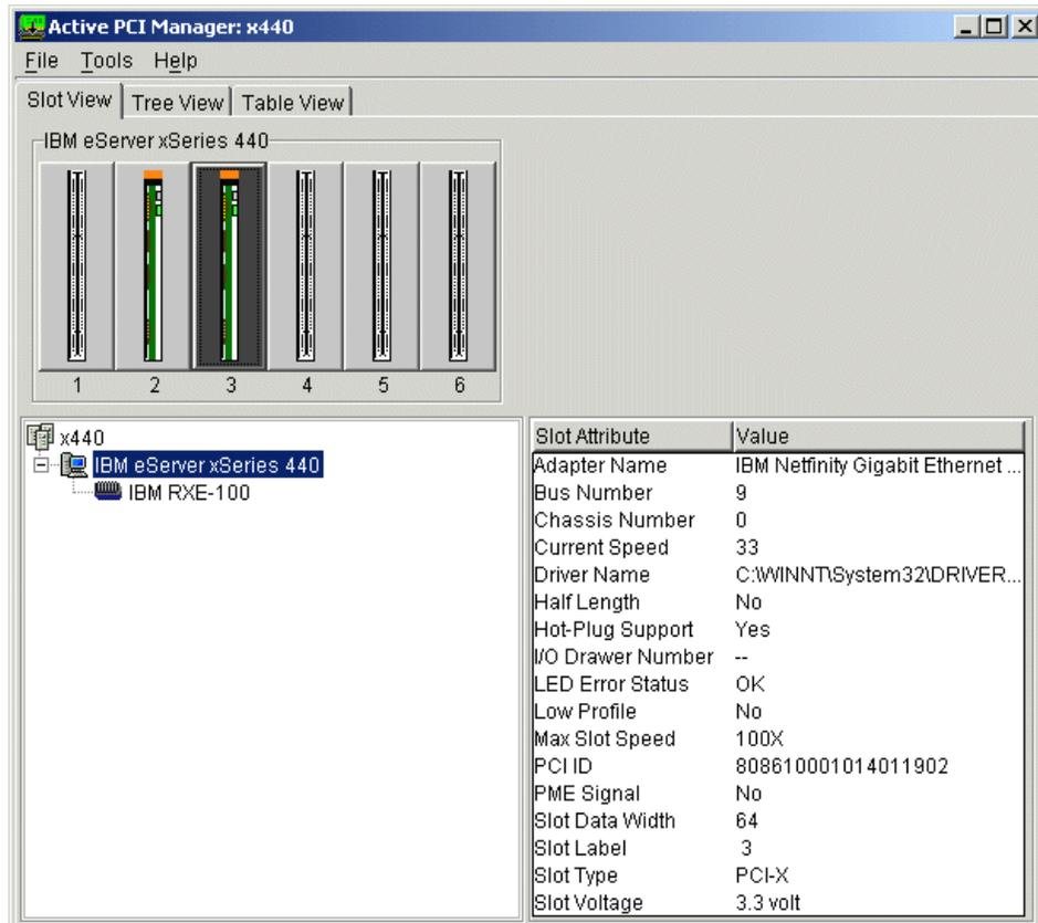
Figure 5-12 IBM Gigabit Ethernet Adapter installed in slot 3
