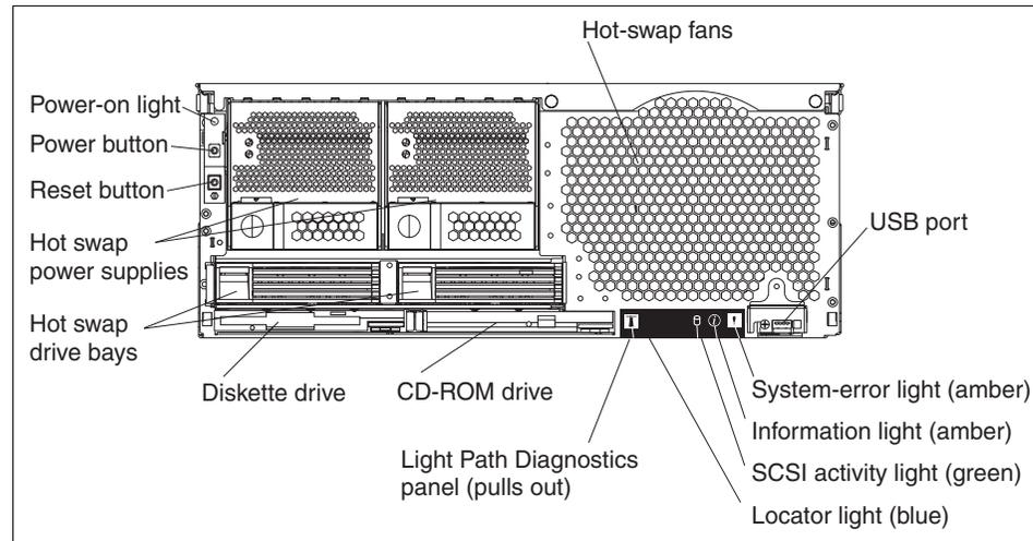
Figure 1-13 Front panel of the xSeries 440
