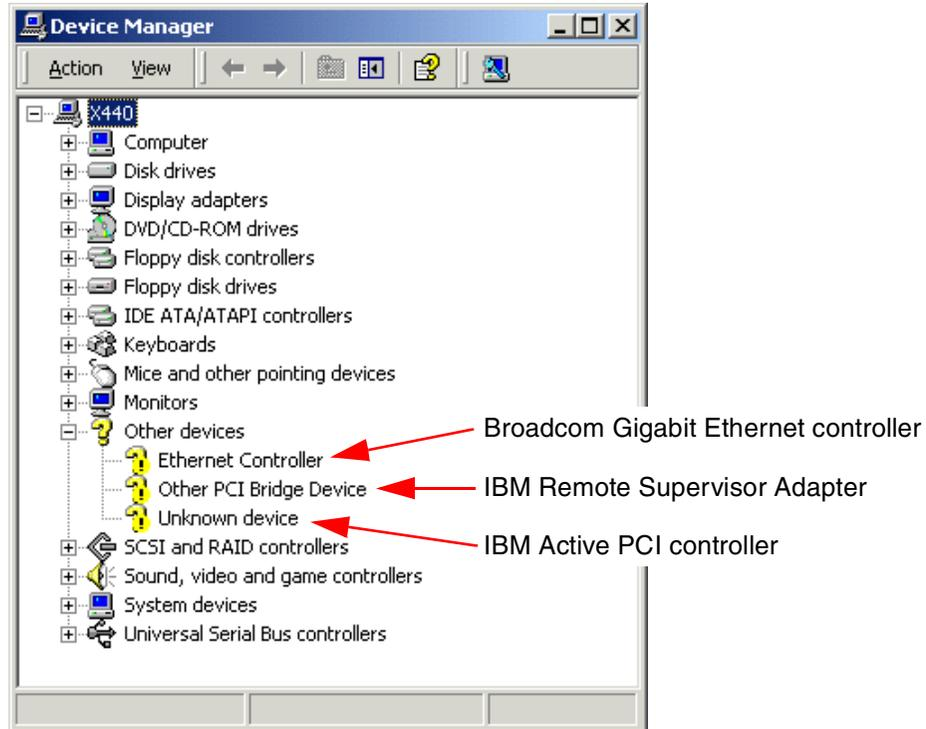
Figure 4-6 Device Manager post Windows 2000 Server installation.
